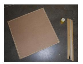
3) Notice how the edges overlap like a pinwheel. This technique allows you to cut all the side sticks the same length.
